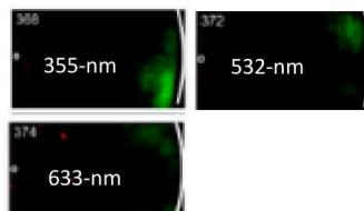
**Initial formation of larger PAH occurs later and farther downstream than smaller PAH, shifting more into the jet-jet interaction regions rather than near the nominal jet axis.**
