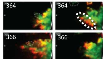
**The spatial distribution of PAH and soot overlap slightly under these threshold-sooting conditions, with soot typically surrounding the PAH. The minimal overlap also suggests that PAHs are rapidly consumed and/or absorbed when soot is formed.**
