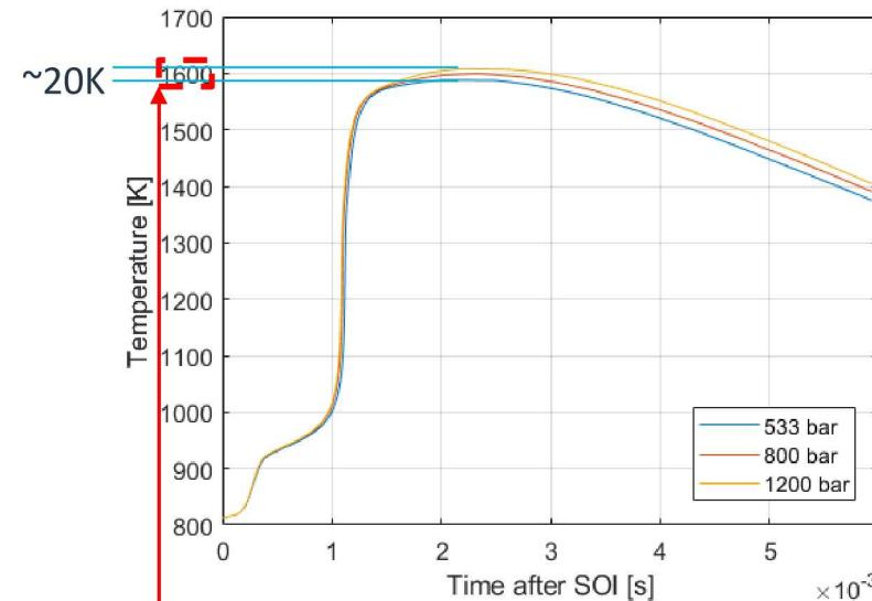
Skeen et.al showed soot formation can vary drastically near a threshold temperature near 1600K within 50 K, which is coincidentally similar to the simulation peak compressed-gas temperature. *Combust. Flame.* 188: 483-487, 2018
