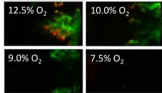
**Increasing dilution delays the inception of PAH as the intake- $O_2$  mole-fraction decreases. Neither larger PAH nor soot are detected with 7.5% intake- $O_2$ . Large PAH appears at 9% intake- $O_2$ , while soot initially appears at 10% intake- $O_2$ .**
