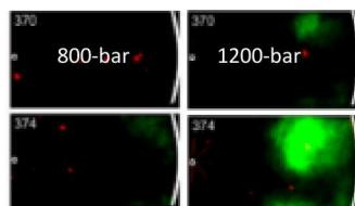
**As the CR fuel pressure is increased from 533 to 800 to 1200 bar at 9% intake  $O_2$ , large PAH first forms at 800 bar, while soot first appears at 1200 bar. This may be explained by increased local temperatures at the higher mixing rates for the higher velocity injection.**
