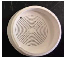
NJ silver & gold ink deposition on alumina
