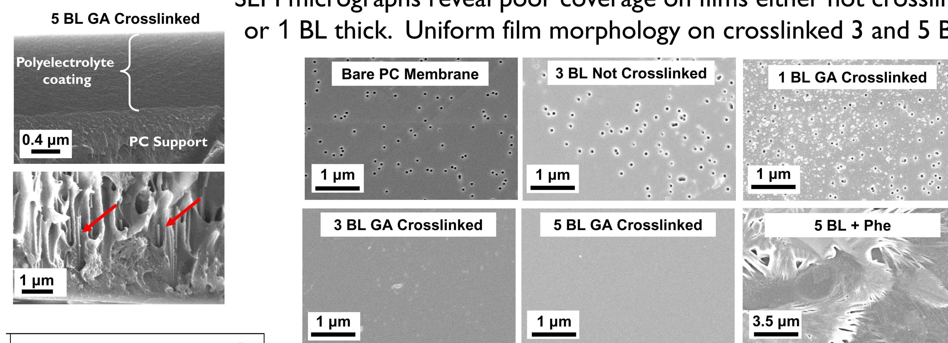
Cross sectional SEM images used to measure polyelectrolyte thicknesses. Thickness increases with number of applied bilayers.
