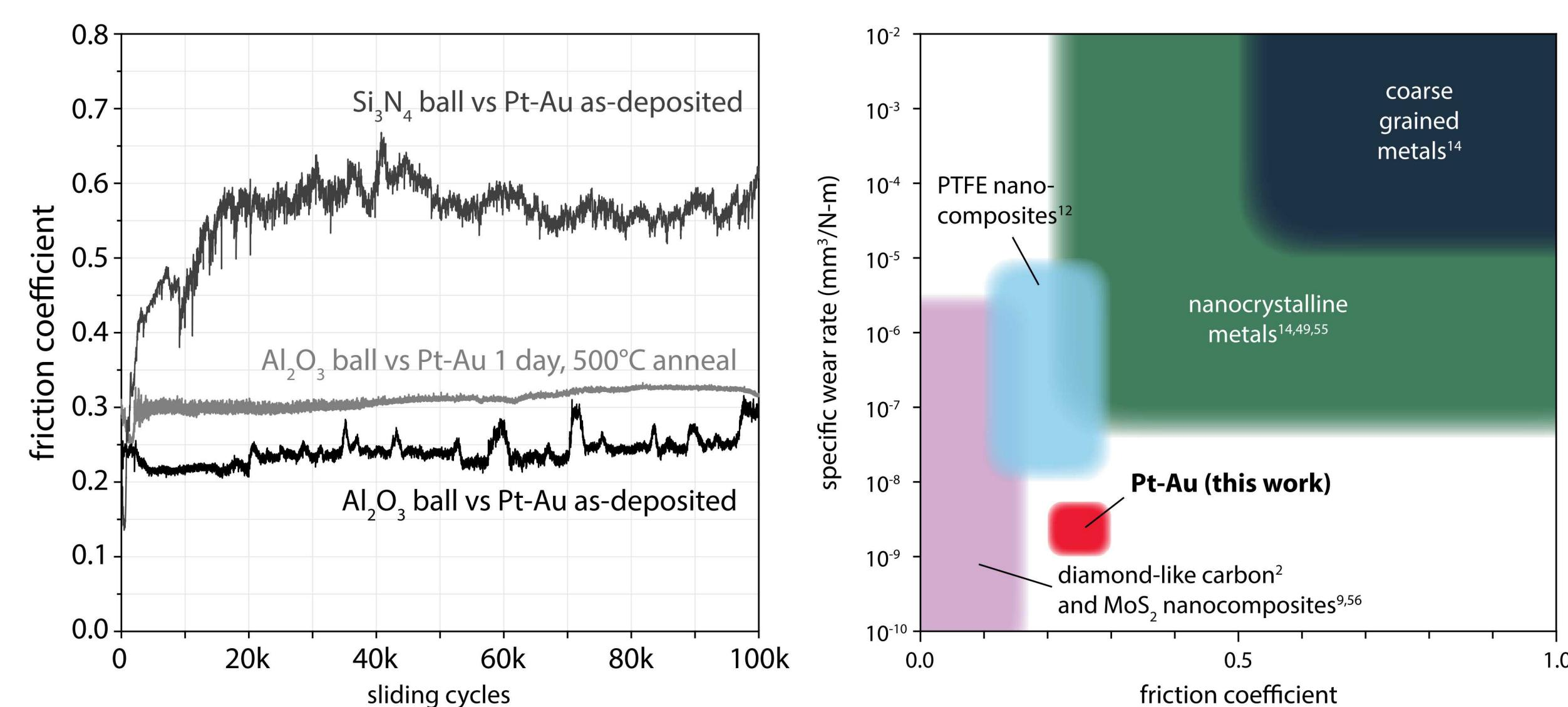
The maximum Hertzian contact stresses of about 1.1 GPa in friction experiments are approximately equal to, or just below, the fatigue endurance limit of these Pt-Au films, and well below the measured nanoindentation hardness of  $7.1 \pm 0.4$  GPa
