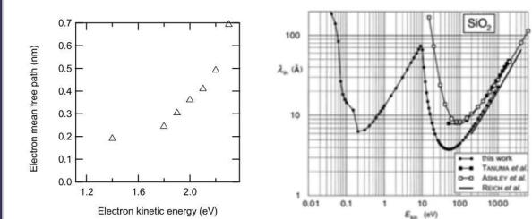
(left) Experimentally-derived photoelectron mean free path as a function of electron kinetic energy. (right) Inelastic mean free path of electrons with kinetic energy  $E_{kin}$  in SiO<sub>2</sub>; the interaction with phonons leads to a second characteristic minimum between the electronic band gap and the phonon energy scales. Reproduced from Kuhn & Fitting, J. Electron. Spectrosc. Relat. Phenom. 105, 257 (1999).
