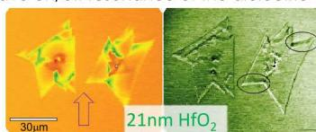
Spatial mapping of cavity mode resonance peak wavelengths and total peak areas. The arrow indicates the in-plane direction of deep-UV sample illumination
