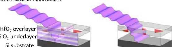
Schematic figures of the sample geometry and the optical standing wave on/off resonance of the dielectric cavities
