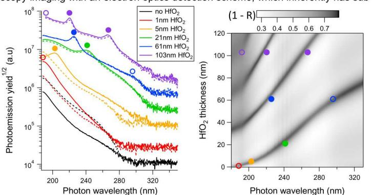
(left) PEY spectra as a function of photon energy obtained at sample locations over MoS<sub>2</sub> flakes (dotted lines) and SiO<sub>2</sub> (solid lines). (right) Total optical absorption (1-R) calculated for dielectric cavities. The solid and open circles depict the positions of resonance peaks in PEY spectra (left).
