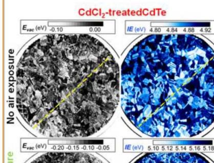
**Grain-to-grain variation** of the vacuum level indicates work function variation. Vacuum level and ionization energy profiles track one another.
