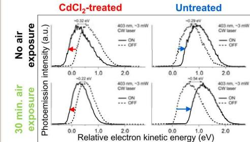
Additional illumination shifted  $E_{\text{vac}}$  to **lower energy** for CdCl2-treated CdTe  $\Rightarrow$  **upward** surface band bending, while  $E_{\text{vac}}$  shifted to **higher energy** for untreated CdTe, indicating **downward** surface band bending.
