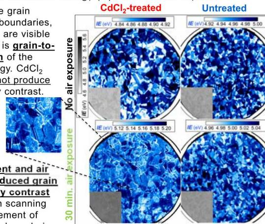
**$\text{CdCl}_2$  treatment and air exposure produced grain (GB) boundary contrast** consistent with scanning probe measurement of activated grain boundaries.
