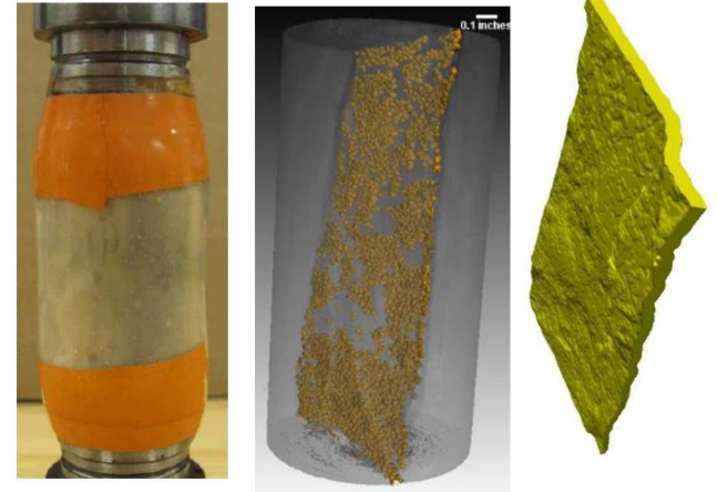
Testing core, rendered image of core, and a view of fracture network (Ingraham et al., ARMA, 2015)
