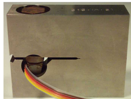
WOL specimen for SCC testing
