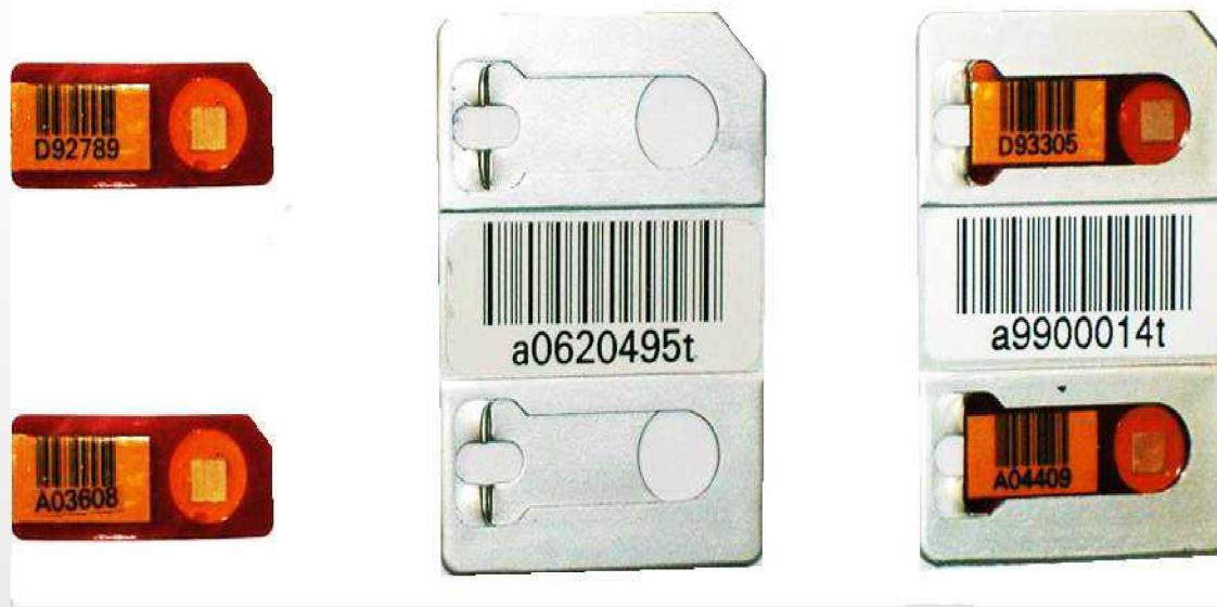
Chipstrates are read using a Harshaw 6600 automatic reader
