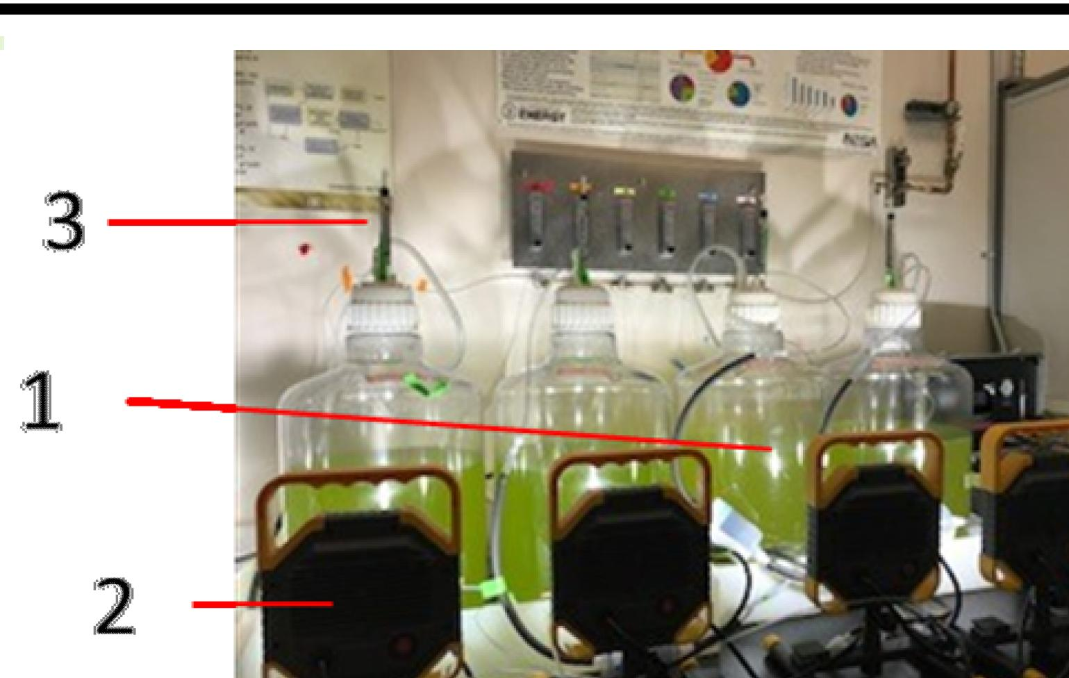
**Experimental Setup:** Growing *N. salina* and *B. plicatilis* cultures (1) with simulated sunlight sources (2) were sampled with SPME fibers (3); VOCs characterized using GC-MS
