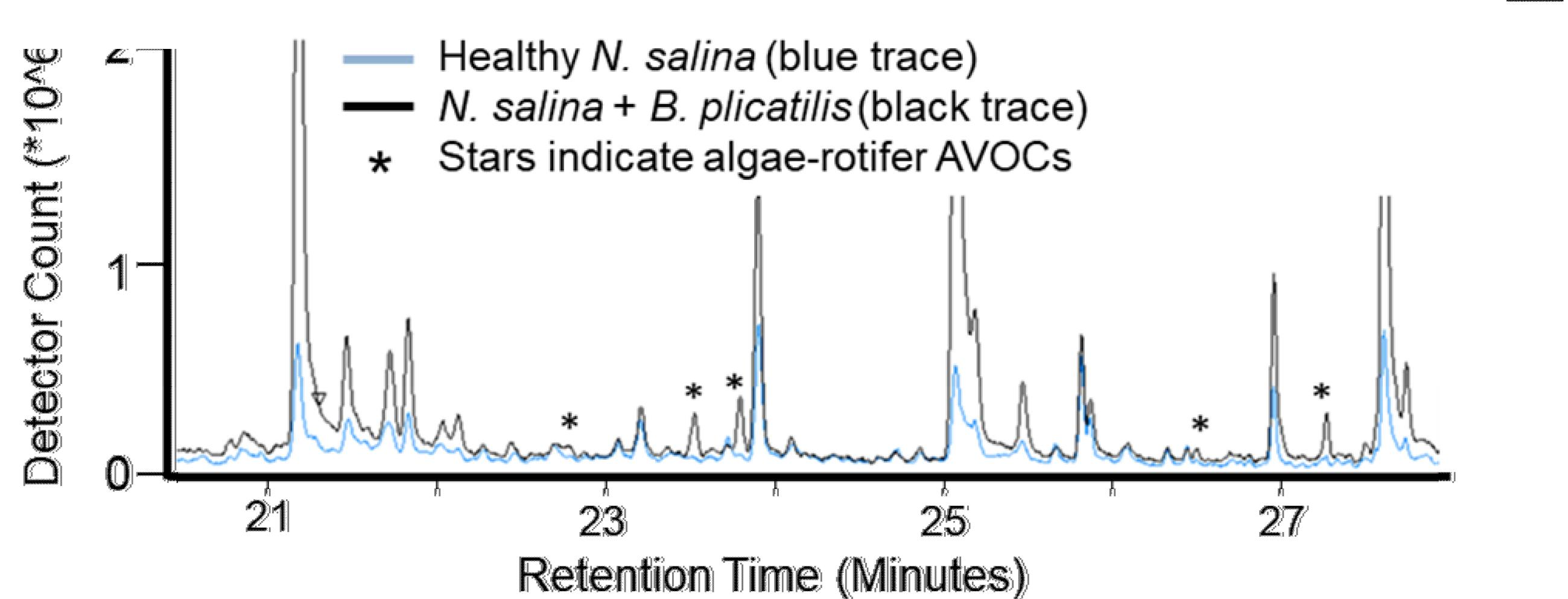
GC chromatogram of AVOCs signals unique to the rotifer-infected cultures, identified through the use of carefully chosen controls (SPME fiber blanks, media blanks, uninoculated algae).
