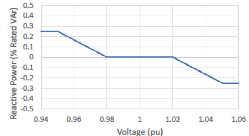
Additionally, a central controller shifts the Volt-Var curve to the right or left based on voltage across the feeder
