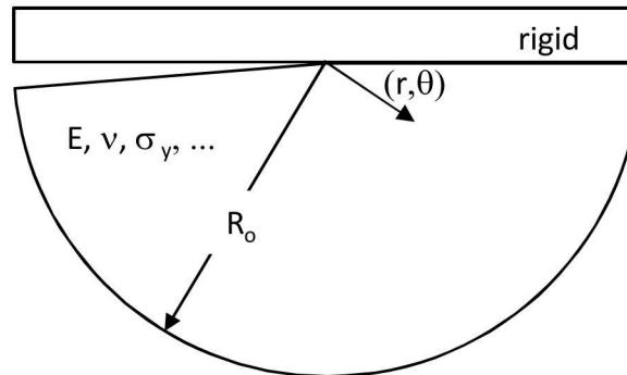
Loading at  $r = R_o$  defined by known linear elastic asymptotic crack tip fields so that it is consistent with a prescribed energy release rate  $G$  and crack-tip mode mixity  $\psi_{r=R_o}$ .
