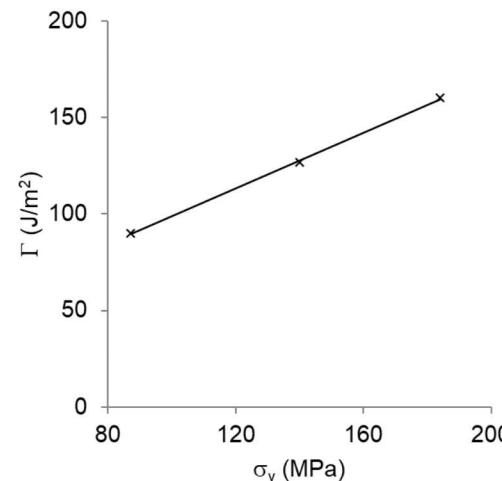
~80 % increase in  $\Gamma$  when test temperature is decreased from 22°C to -65°C ( $R_q = 4 \mu\text{m}$ )
