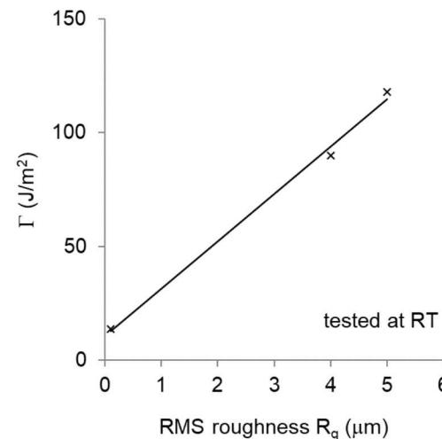
> factor of 9 increase in  $\Gamma$  when  $R_q$  is increased from 0.1  $\mu\text{m}$  to 5  $\mu\text{m}$  (tested at 22°C)
