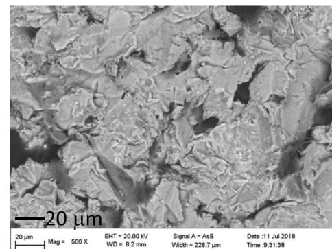
Note: backscatter SEM images. Used EDS to identify al/epoxy regions. Then image thresholding where black=> carbon
