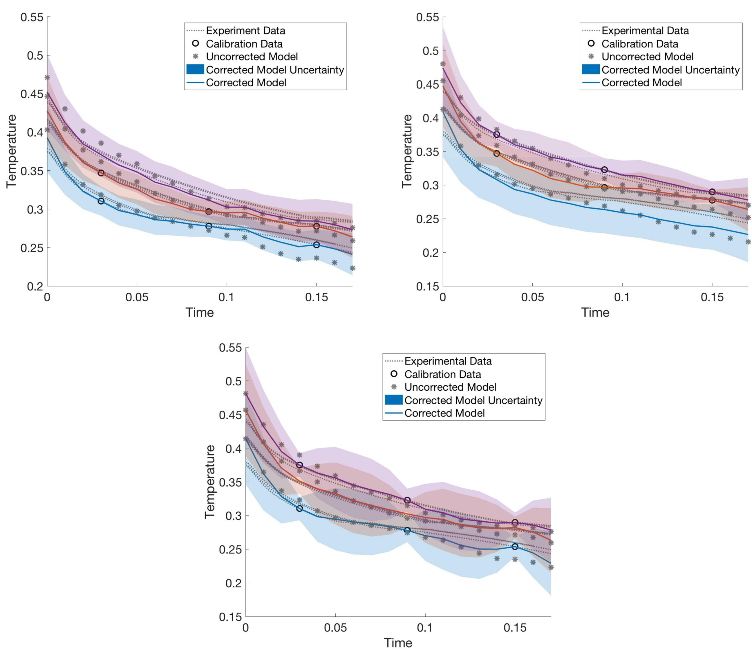
Discrepancy model corrected some areas better than others, but experimental data is contained within the prediction intervals of the corrected model
