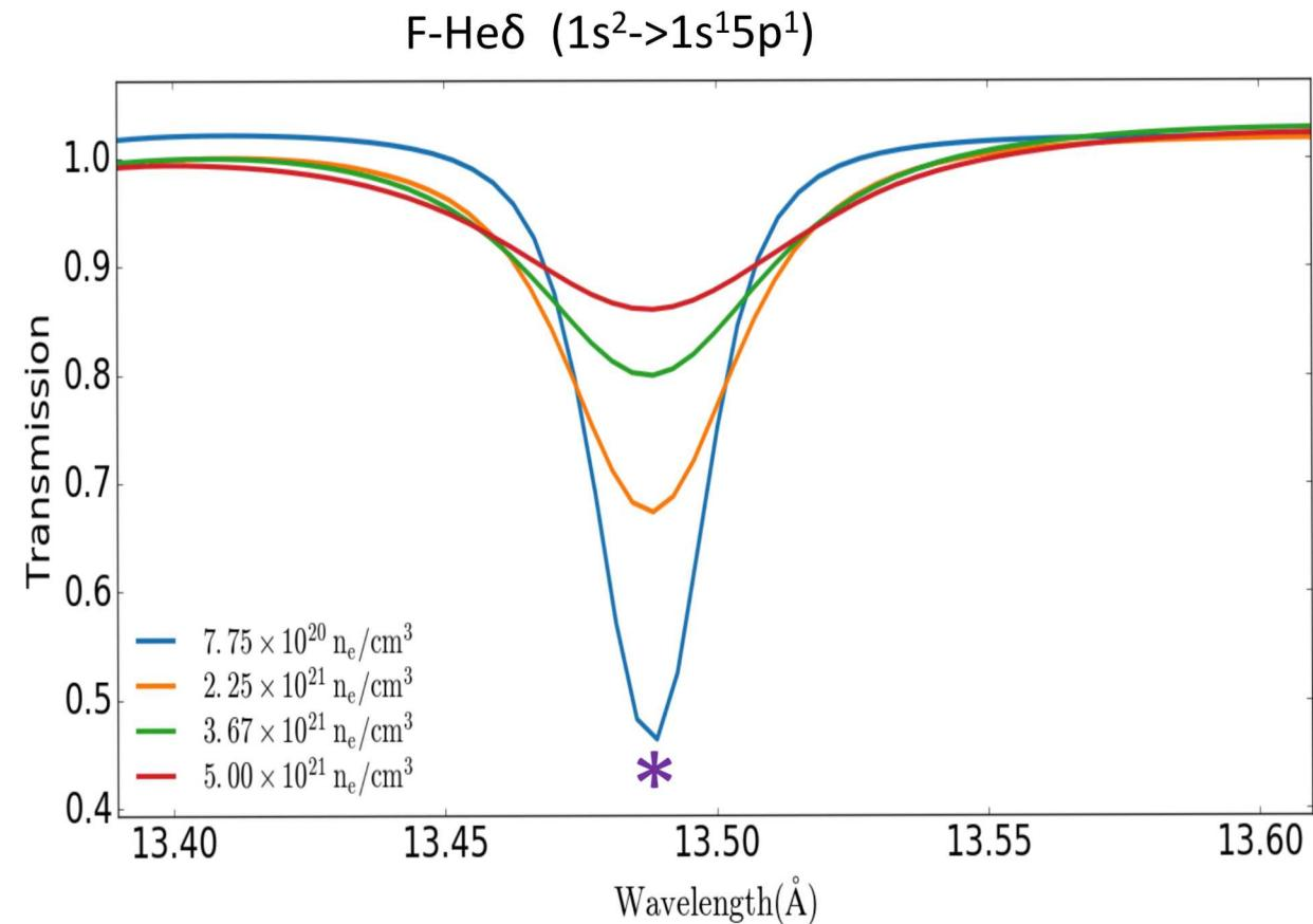
Even the smallest electron density shown here has the width of the line as  $\sim 20 \text{ m}\text{\AA}$ , well above our instrument resolution
