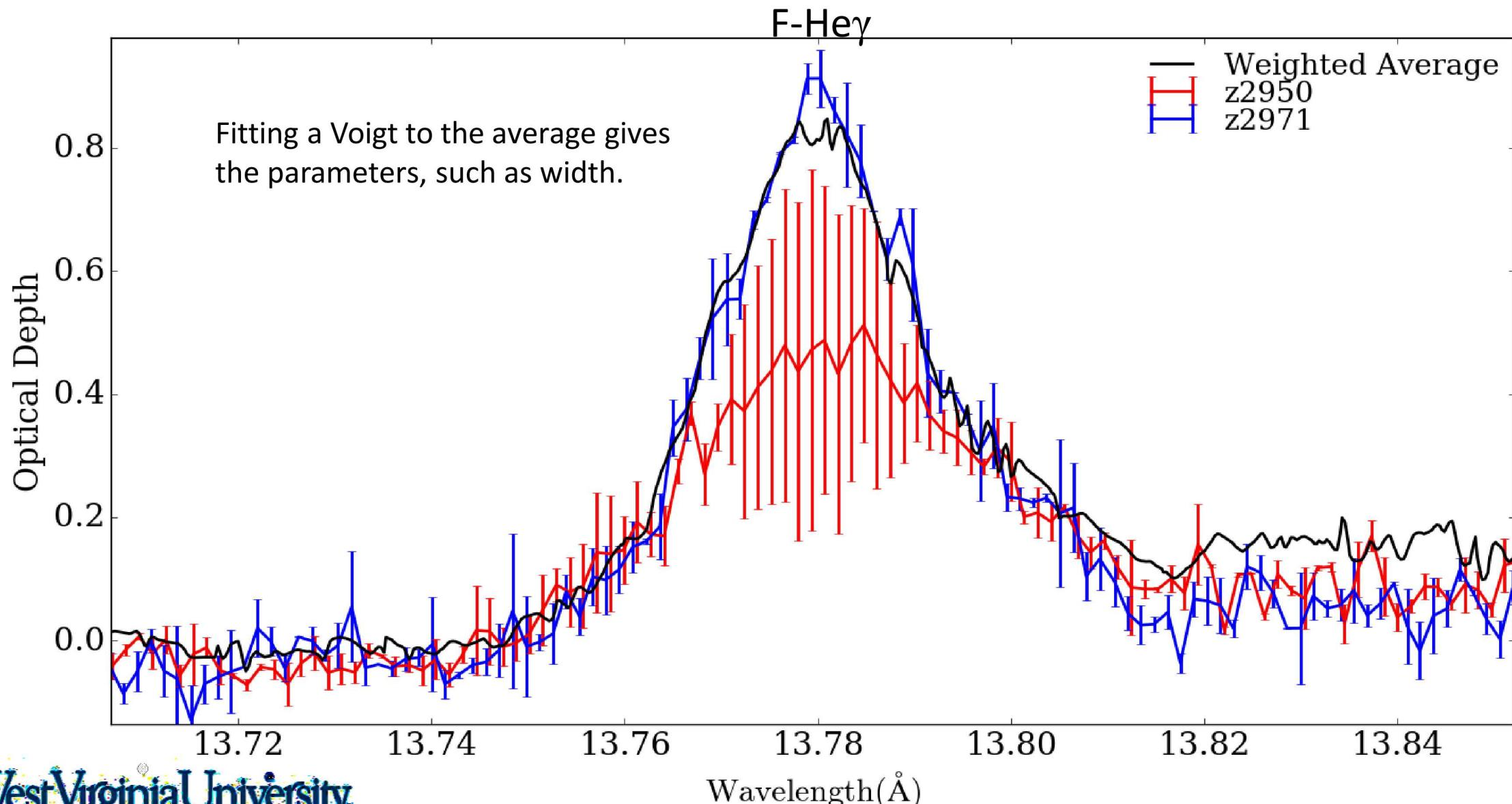
Determining electron density from spectra
