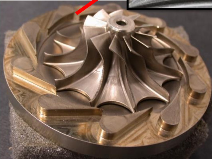
Image: Sandia turbine assembly. Inset shows damage to nozzle after operation with s\text{CO}_2 [1].
