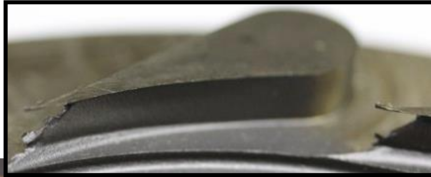
Image: Sandia turbine assembly. Inset shows damage to nozzle after operation with s\text{CO}_2 [1].
