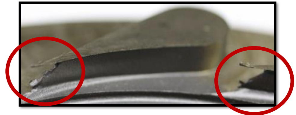
FIG: Eroded nozzle at SNL
