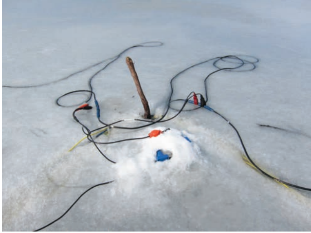
Figure 6. Photo of the northwest vertex of the array showing poor cable-to-ice coupling, ( i.e. , the yellow fiber-optic cable was loose in the air), which will give poor first arrivals.
