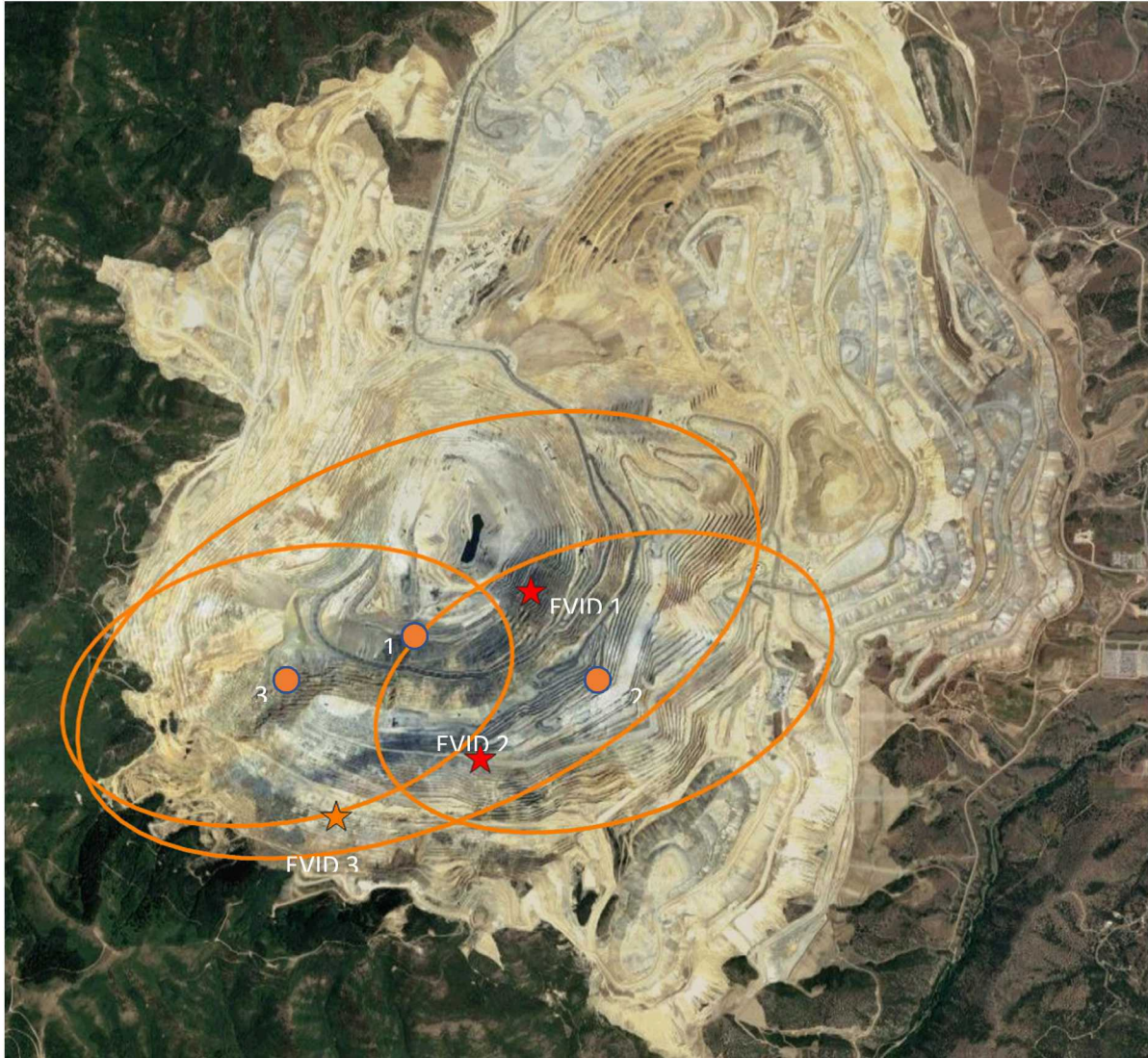
Figure 8. Event relocations of 3 GT events at Bingham Mine with 95% coverage ellipses. GT events are shown as red stars and labeled from top to bottom as EVID 1,2, and 3, respectively. Relocations performed using our model are shown as orange dots. Each event is labeled by their corresponding GT event ID (e.g., event 1 corresponds to EVID 1).
