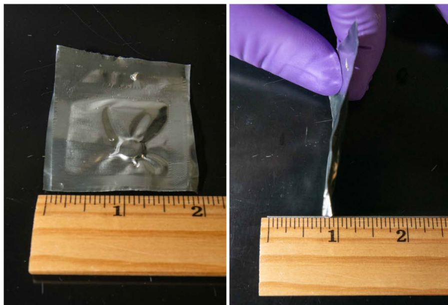
Figure 2: Steel coupons heat-sealed inside sample pouches. See text for discussion of sealing conditions.
