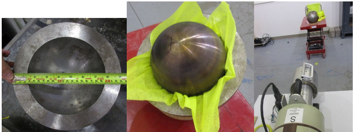
Figure 8. The nested DU sphere and shells surrounded by 1.25 inches of iron
