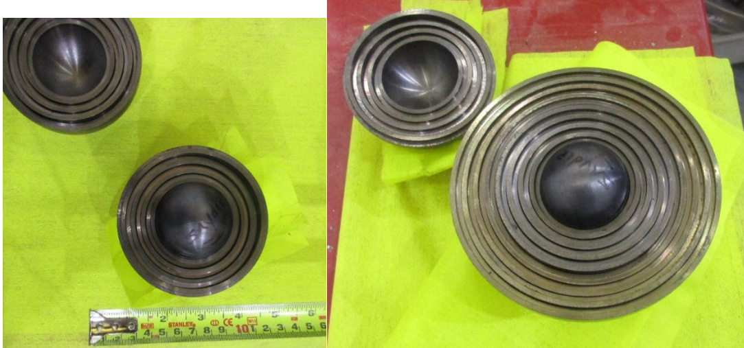
Figure 7. Sphere and nesting shells of DU to make 4 inch and 6 inch spheres
