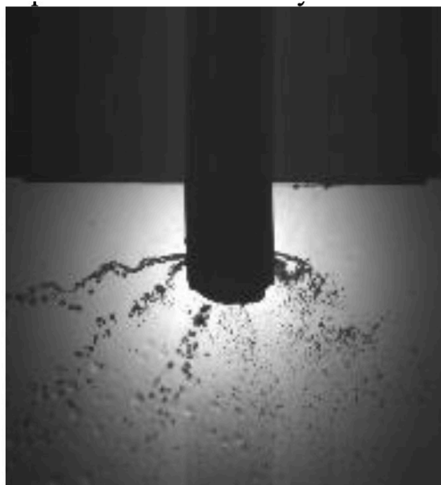
Figure 117 Typical Jet Atomization (No even distribution of gaseous flow is seen)
