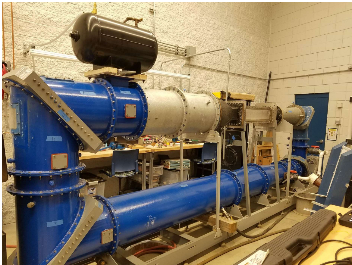
Figure 33. High-Speed cavitation tunnel (HiCaT): in its new home in 176 Chase Ocean Engineering Lab.
