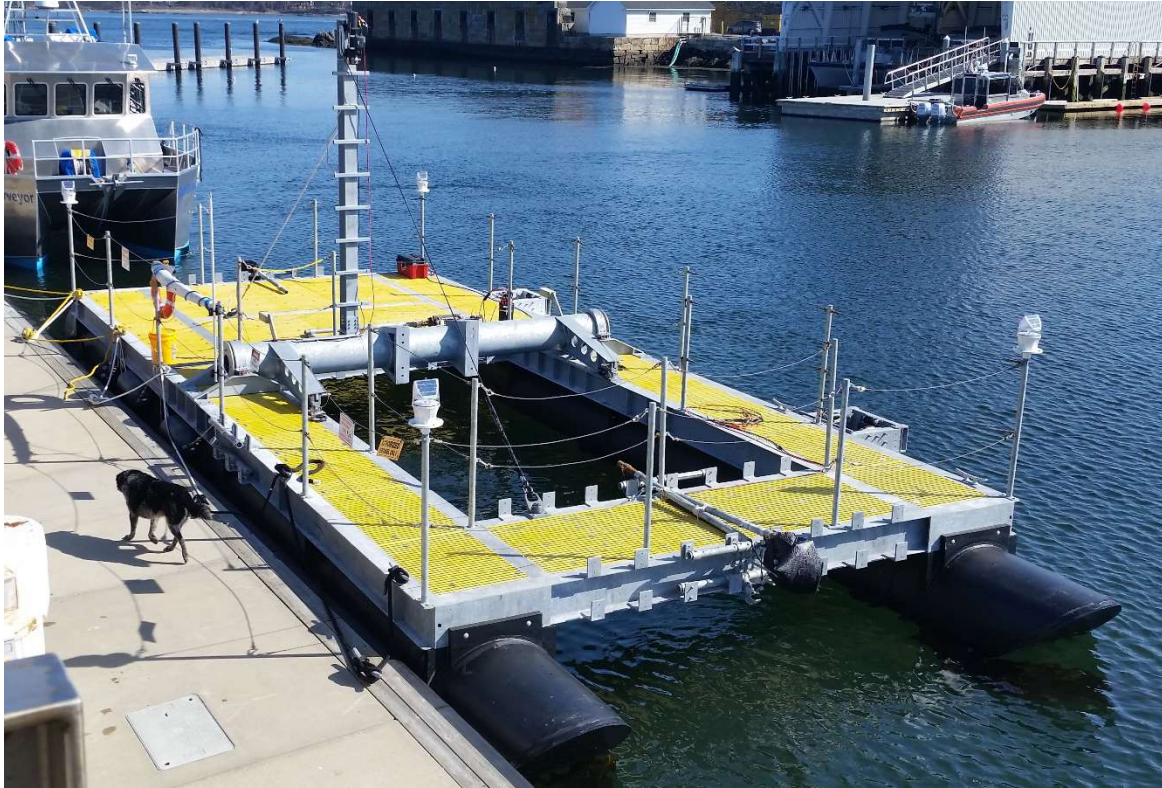
Figure 3. Department of Energy (DoE)-funded Turbine Deployment Platform (TDP). built and deployed TDP system at UNH Pier, prior to installation of the first hydrokinetic turbine.
