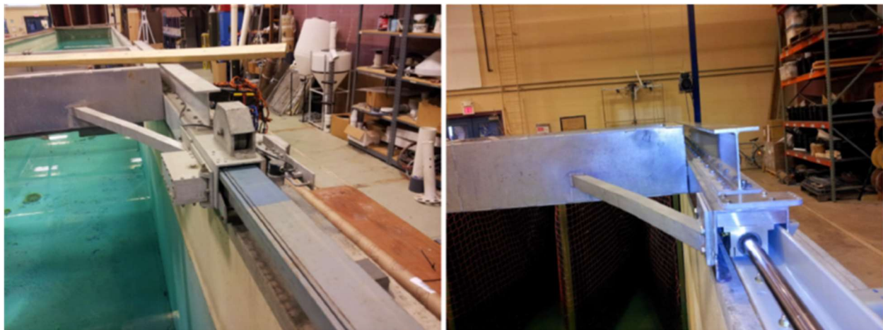
Figure 17. Comparison of old (left) and new, upgraded (right) linear guide system on the “master” side of the tank.
