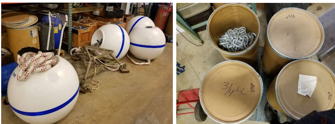
Figure 8. Components of mooring system for Tidal Energy Test Site at General Sullivan Bridge. Left: buoyancy floats and pennants, right: \frac{3}{4} " galvanized steel chain (currently in storage in Chase Ocean Engineering Laboratory).
