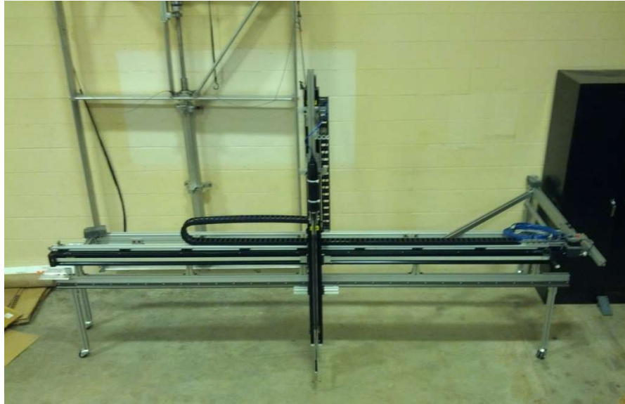
Figure 21. UNH towing tank 2-axis traversing system shown in Figure 20, as built.
