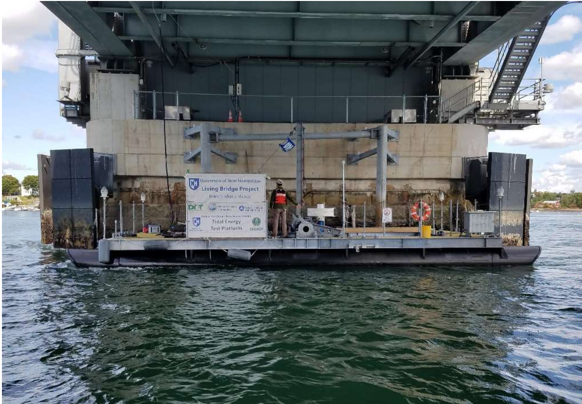
Figure 13. Tidal Turbine Deployment System at the Memorial Bridge in Portsmouth, NH including the Vertical Guide Posts anchored to Pier #2 and the Turbine Deployment Platform.
