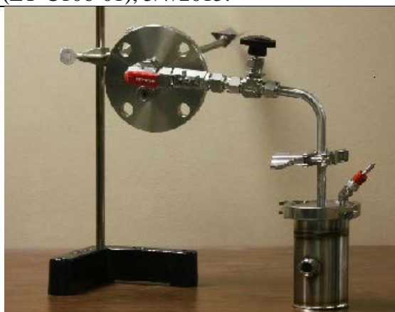
Exhibit 4.9.3. Column Liquid/Gas Sample Collection Port.
