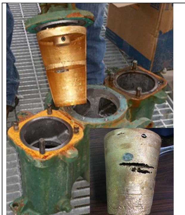
Exhibit 6.4.9. Corroding amine strainer fabricated materials not specified for amine service that was removed after the conclusion of the MEA solvent testing campaign.
