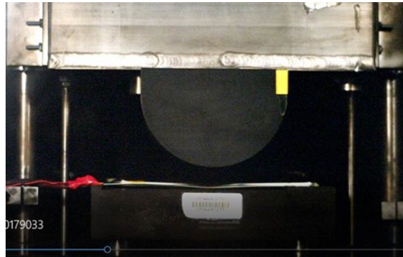
Figure 8: Still image of a high-speed video from impact testing, where a pouch cell is impacted by a semi-cylinder indenter.
