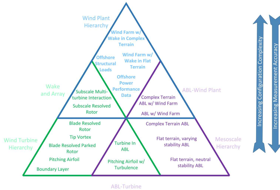
Figure 4-2. Validation studies mapped to the wind plant performance validation hierarchy.
