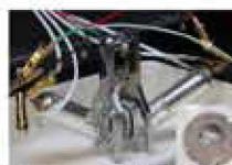
Symmetric cell with MMT separator (Sn-coated) before and after cycling
