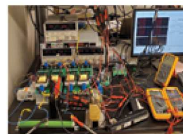
Figure (10). Hardware set up for open circuit voltage calculation of a BM
