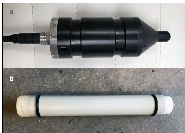
Figure 10.2. Examples of a “conventional” PAM instrument (Ocean Instruments NZ SoundTrap ST300 HF) (a) and a “stand-alone” PAM instrument (b). (Photos courtesy of Daniel Hasselman)
