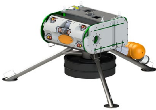
Figure 10.10. The Adaptable Monitoring Package (AMP). An integrated subsea instrument package developed by the University of Washington that is used to monitor marine renewable energy devices. (Image courtesy of Applied Physics Laboratory, University of Washington)
