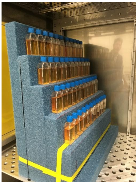
Fig. 12. Modified incubator for use in beamline with holder that can accommodate up to fifteen T75 flasks in a 3 by 5 array or forty four T25 flasks. Panel a) modified incubator; Panel b) holder for T25 flasks.
