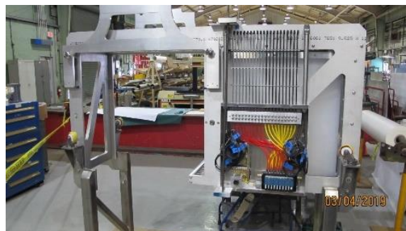
Fig. 19. Large binary filter system installed in NSRL beam line.
