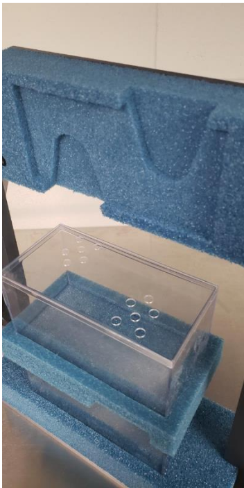
Fig. 11. Ventilation lids for air circulation. The non-ventilated sides of the lids are painted red to serve as a quick visual cue that the lids are in the correct orientation for air flow.
