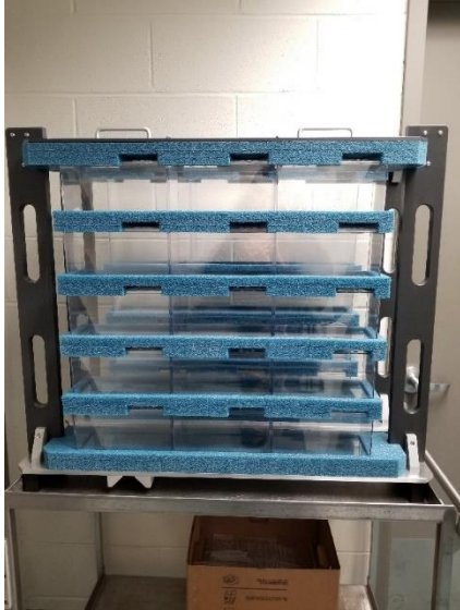
Fig. 9. Cage array for mouse irradiations in the 60 by 60 cm 2 beam.
