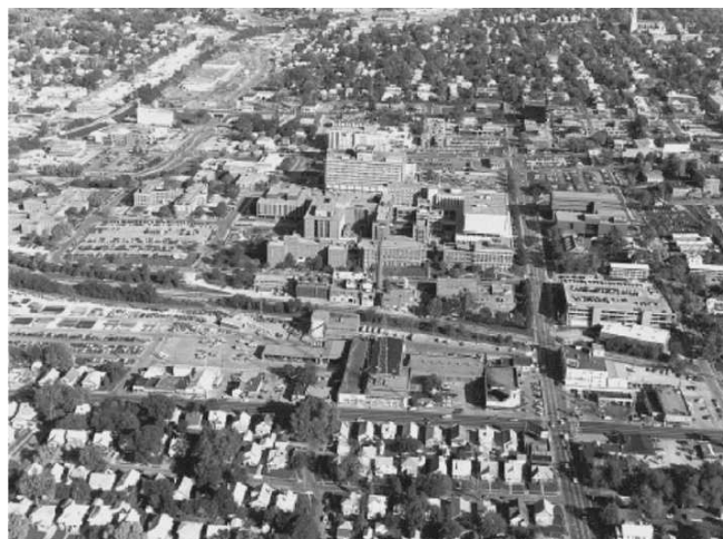
FIGURE C26.7-5(b) Exposure B: Urban Area with Numerous Closely Spaced Obstructions Having the Size of Single-Family Dwellings or Larger. For All Structures Shown, Terrain Representative of Surface Roughness Category B Extends More Than 20 Times the Height of the Structure or 2,600 ft (792 m), Whichever Is Greater, in the Upwind Direction.
