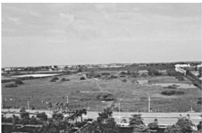
FIGURE C26.7-6(a) Exposure C: Flat Open Grassland with Scattered Obstructions Having Heights Generally Less Than 30 ft (9.1 m).
