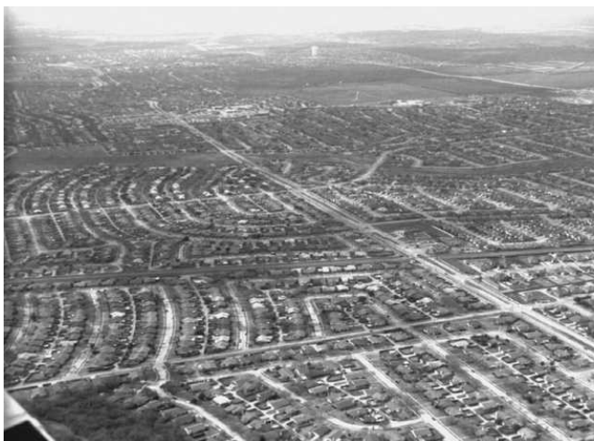
FIGURE C26.7-5(a) Exposure B: Suburban Residential Area with Mostly Single-Family Dwellings. Low-Rise Structures, Less Than 30 ft (9.1 m) High, in the Center of the Photograph Have Sites Designated as Exposure B with Surface Roughness Category B Terrain around the Site for a Distance Greater Than 1,500 ft (457 m) in Any Wind Direction.
