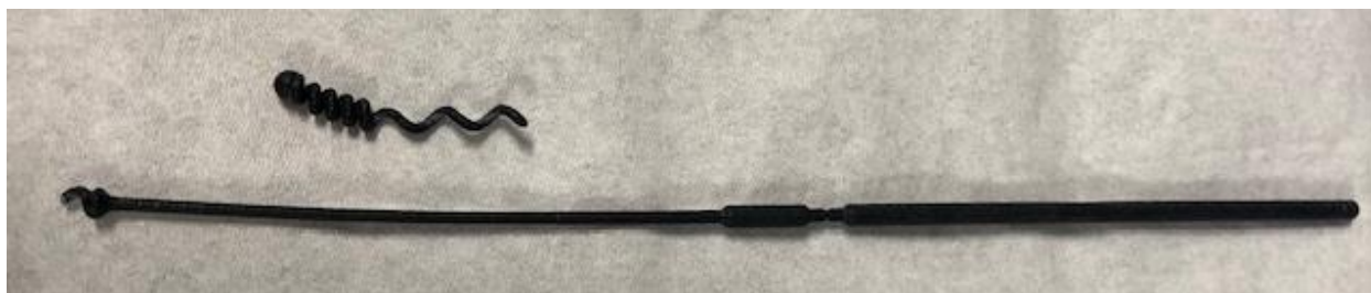
Figure 26. Representative image of a swab classified as breaking at the “Head-Neck.”
