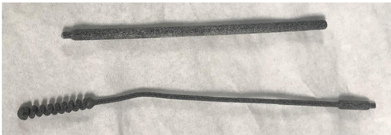
Figure 28. Representative image of a swab classified as breaking at the “Breakpoint.”
