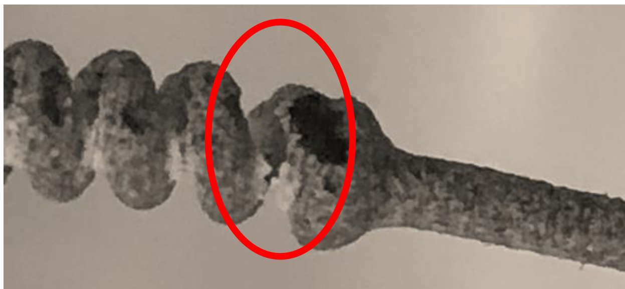
Figure 27. Representative image of a swab classified as breaking at the “Head.” The break location is shown circled in red in the bottom image. In many cases, though, the actual break location was not visually observable and the swabs were classified as having broken based on the force-elongation data.
