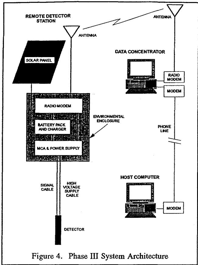
Figure 4. Phase III System Architecture
