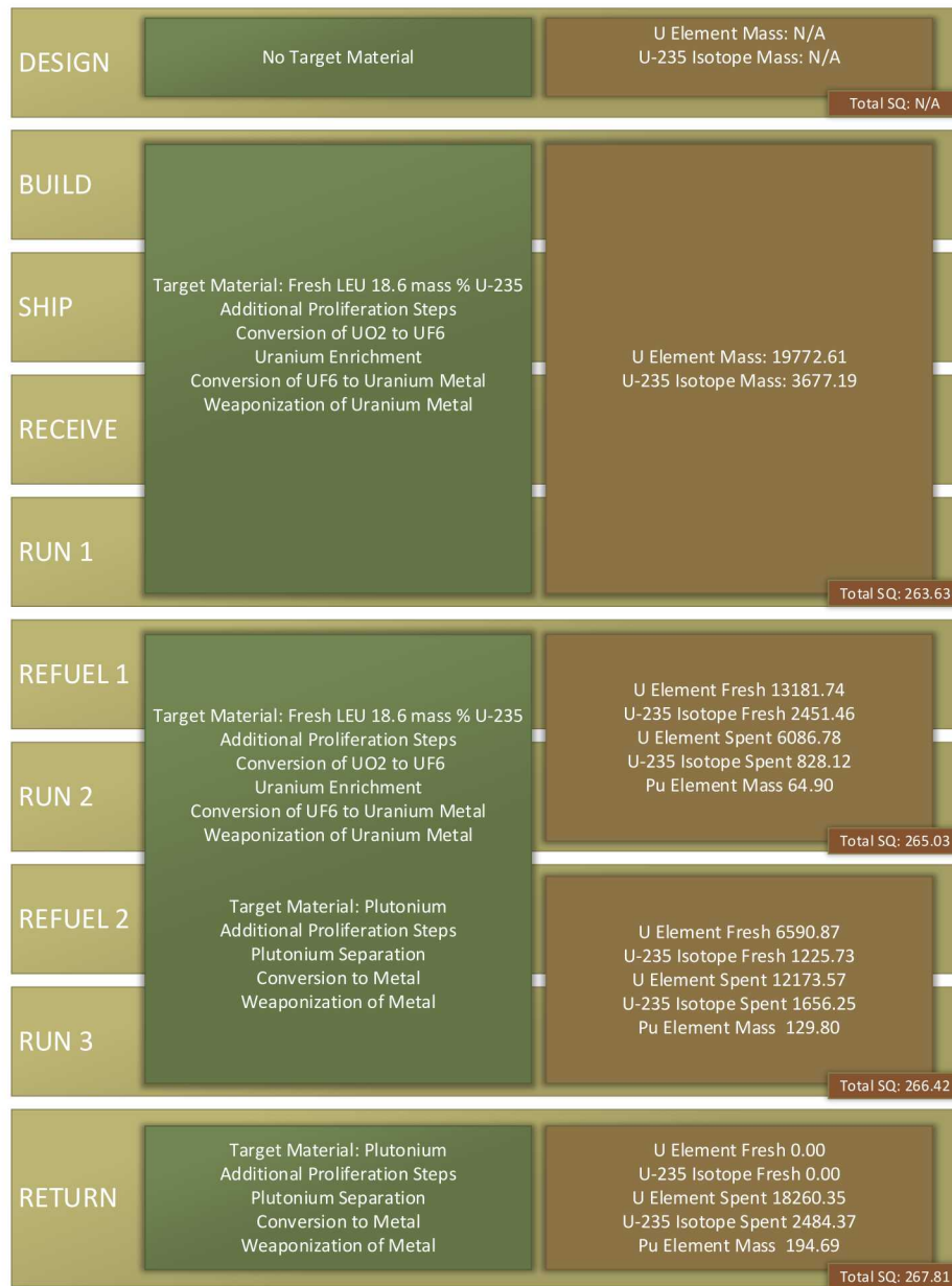
Figure 4. Nuclear Material Constituent Process Flow through the FNPP Operational Lifecycle Stages (all mass quantities in kilograms)
