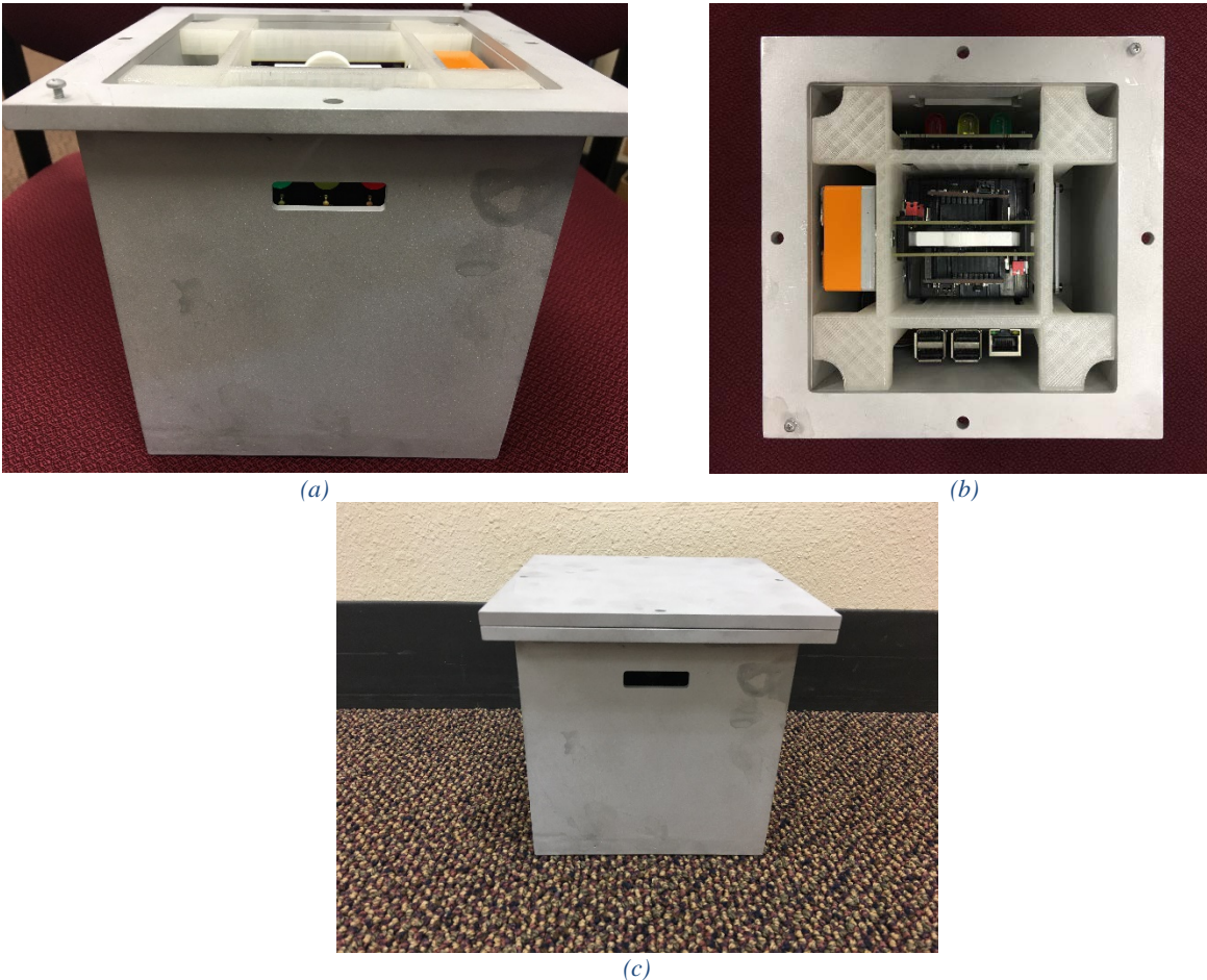
Figure 5: Buddy Tag Enclosure. (a) Side view showing the opening for the window and openings for the hasp seal. (b) Top view showing the Buddy Tag placed within the enclosure. (c) Side view showing the top in place on the enclosure.
