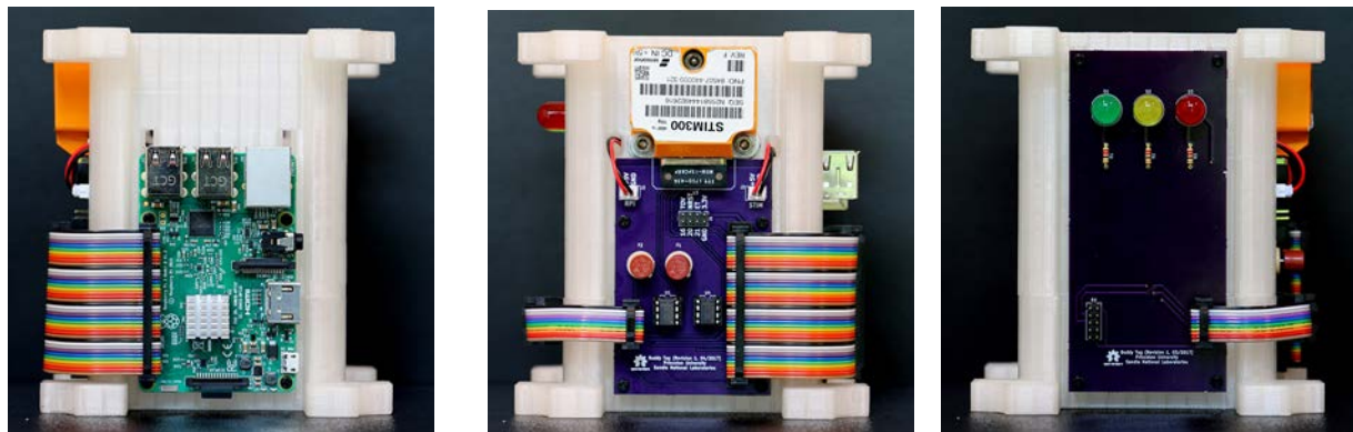
Figure 4: Buddy Tag Modules. The module with the inertial measurement unit (left) forwards the incoming data to the GPIO pins of the Raspberry Pi 3 located on a separate module (middle), where a dedicated algorithm processes the data in real-time. Results are displayed via the output module (right).[7]
