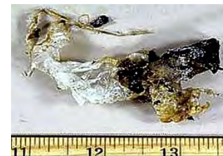
A) Semtex 1A (87% PETN with dye, antioxidant, plasticizer, and binder)
