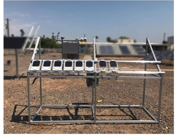
Fig. 3. NOCT test rack and single-cell coupons installed in Mesa, Arizona, USA. (Coupon identification from left to right: TCB-A, TCB-A, TCB-B, TCB-B, TPT, TPT, glass/glass, and glass/glass)
