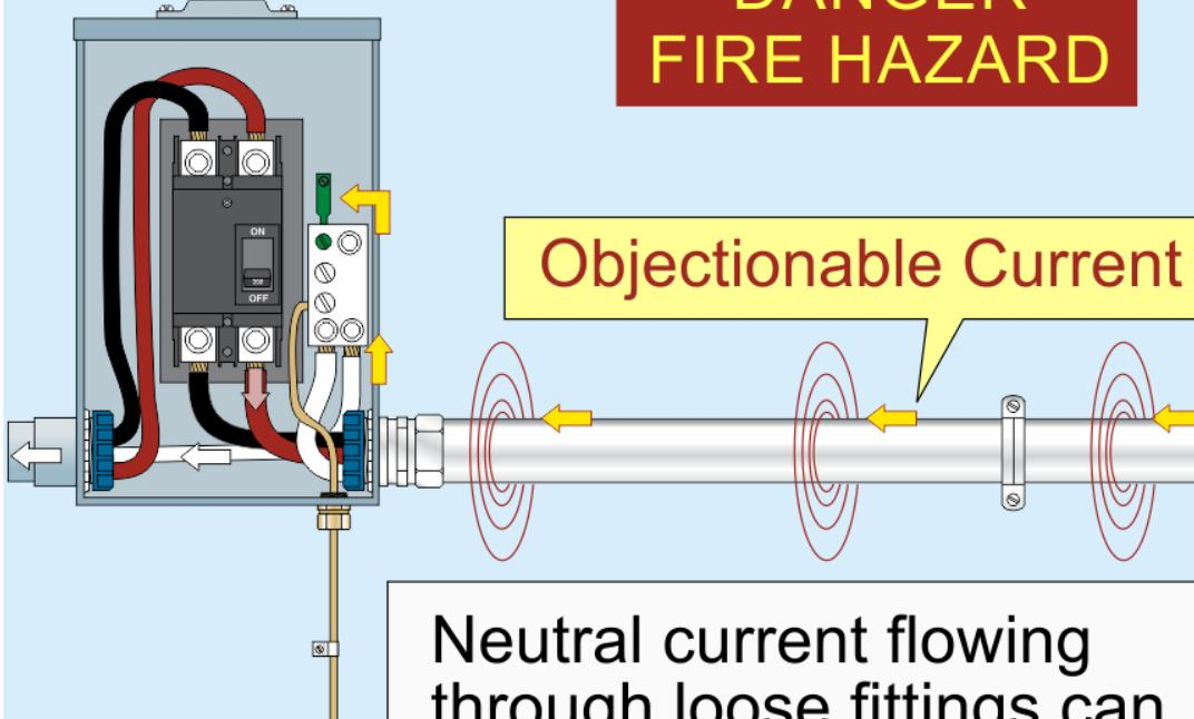
Neutral current flowing through loose fittings can cause the temperature to rise, igniting surrounding combustible materials.
