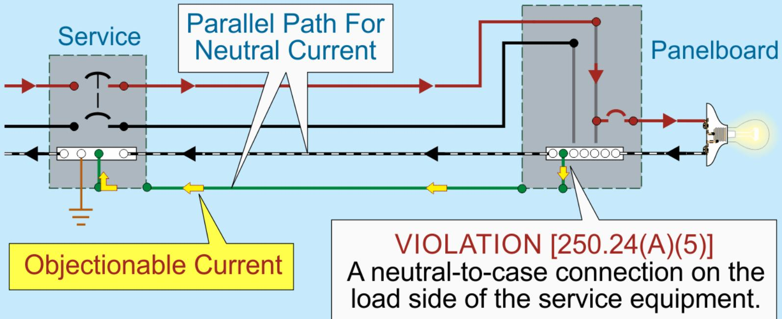
Objectionable neutral current will flow on the equipment grounding conductor when the neutral conductor is connected to the metal case of a panelboard on the load side of service equipment.
