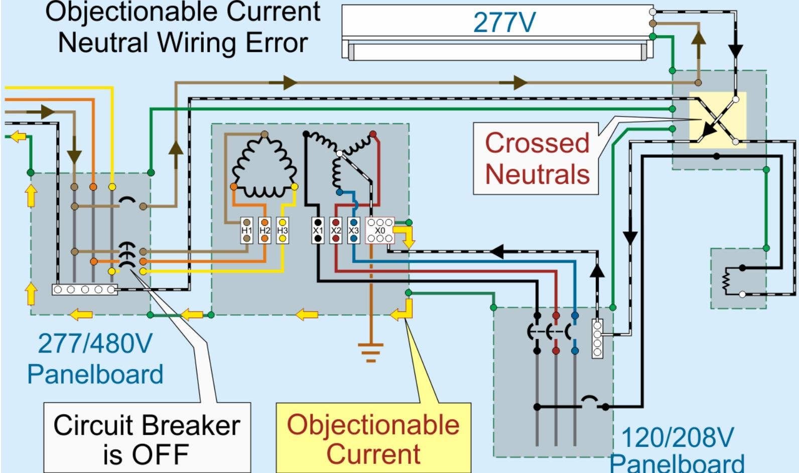
**DANGER:** The 120/208V panelboard (de-energized) can have dangerous voltage from the 277V lighting circuit because of the crossed neutrals.
