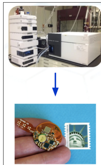
Figure 3.4.2. Development of high-performance liquid chromatography on a chip. (Courtesy of C. Stafford, NIST.)
