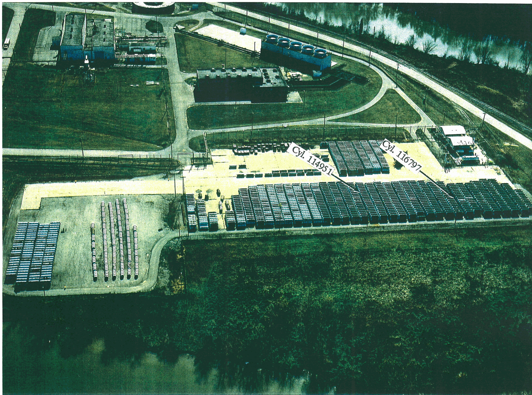
Fig. 2. K-1066-E yard. Photograph illustrates locations of failed Cylinders 114951 and 116797. Note the path of rust from breached Cylinder 114951.
