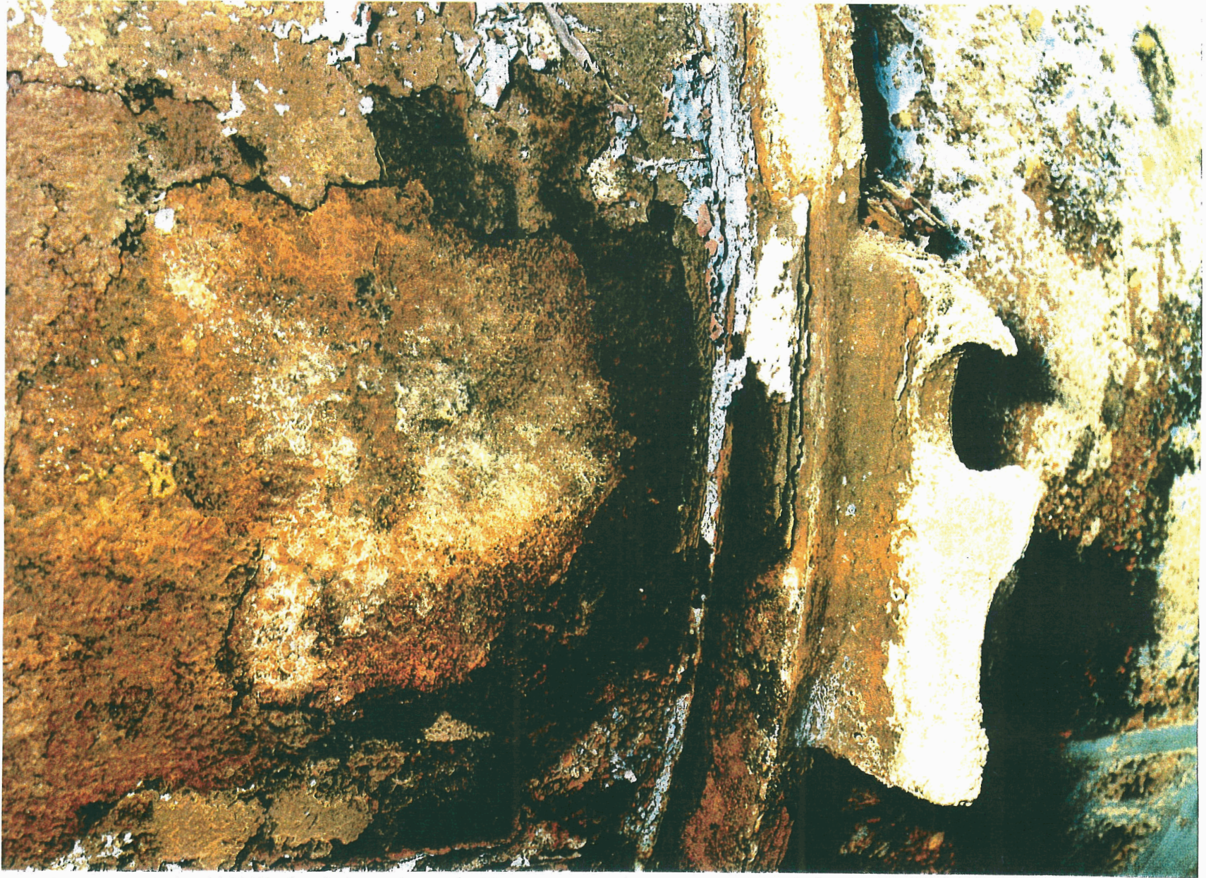
Fig. 5. Cylinder 115017 after being relocated. Note the extensive wastage of the lifting lug. This lug is believed to have impacted and caused the breach in Cylinder 114951. Also note the cylinder wall wastage - an effect of corrosive materials released from breached Cylinder 114951.
