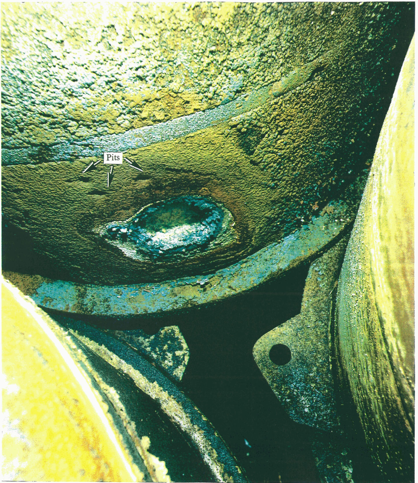
Fig. 3. Breached Cylinder 101244 in stacked position as discovered. Note the three significant pits between the breach and the cylinder head weld.
