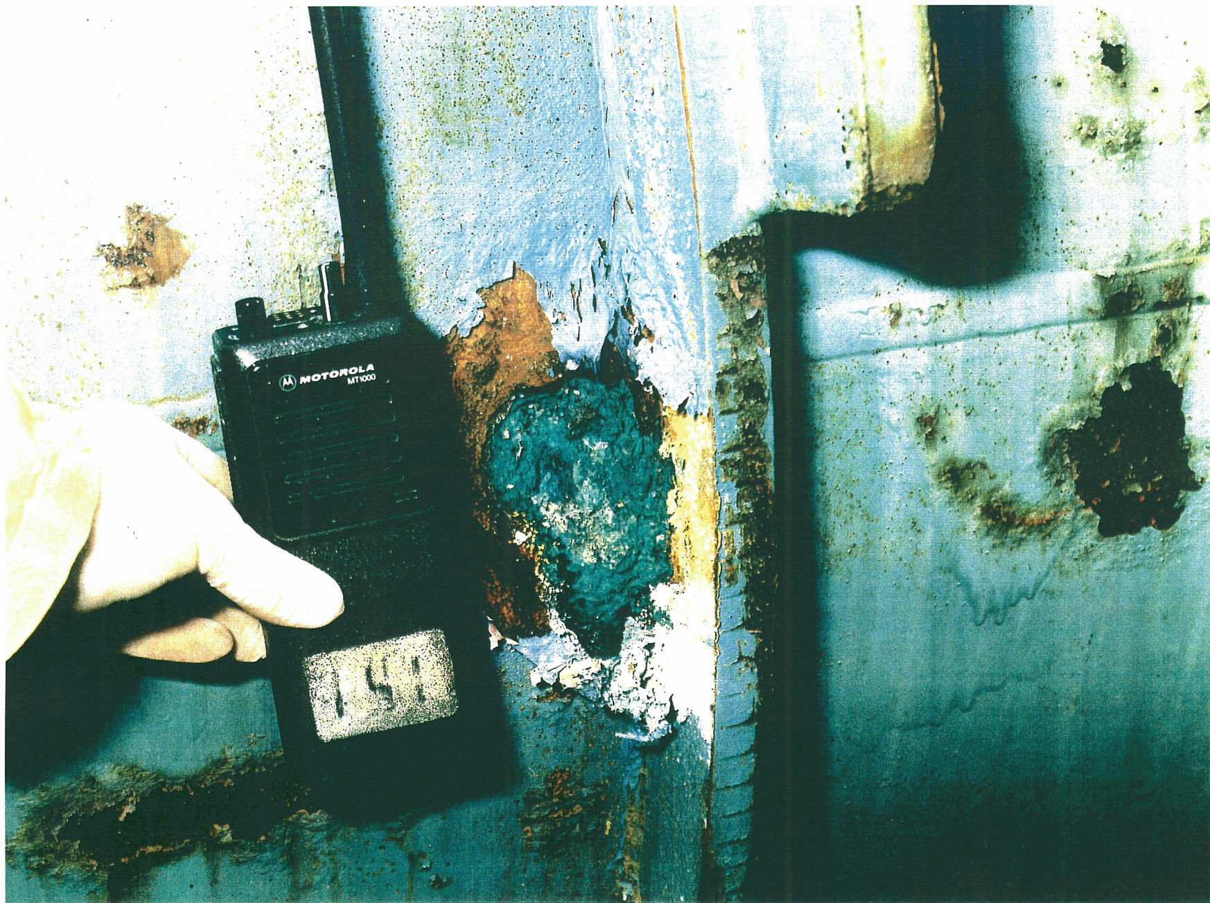
Fig. 7. Breached Cylinder 116797. Photograph taken after neighboring cylinders were relocated.
