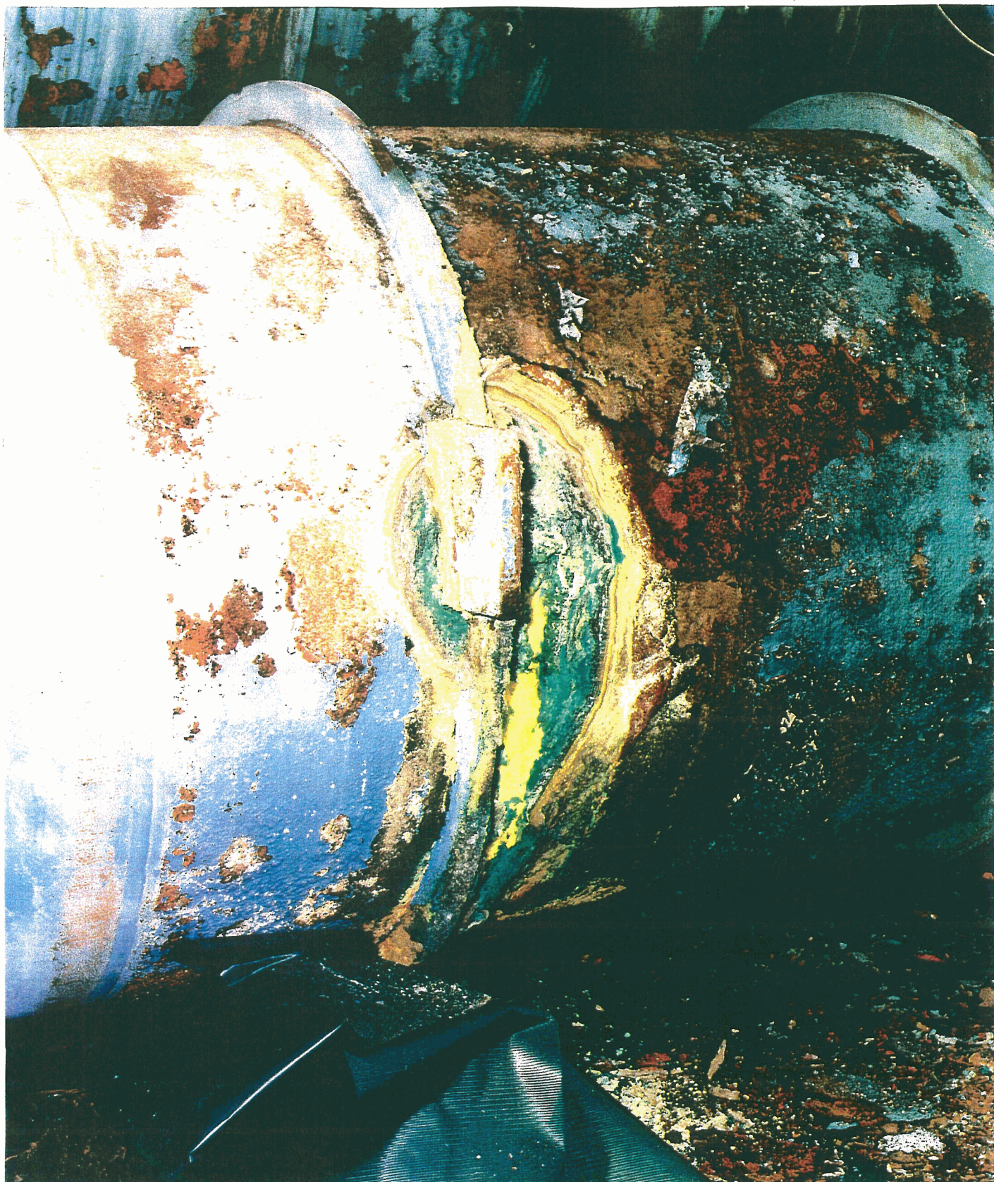
Fig. 4. Breached Cylinder 114951 after neighboring cylinders have been relocated.
