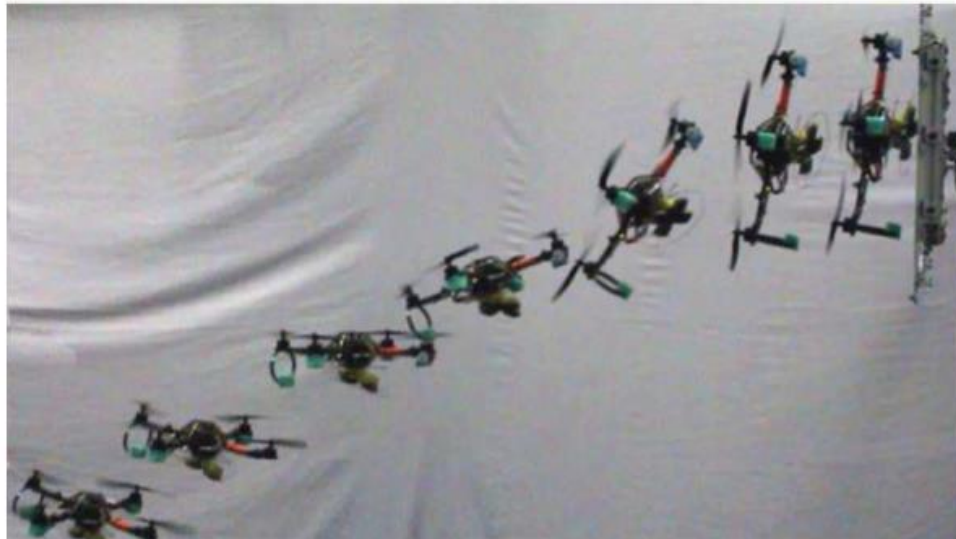
Figure 11) Many research organizations have shown how to "perch" a quadcopter onto a wall or ceiling. This image from the University of Pennsylvania demonstrates a perching maneuver that allows the quadcopter to stick to a wall.
