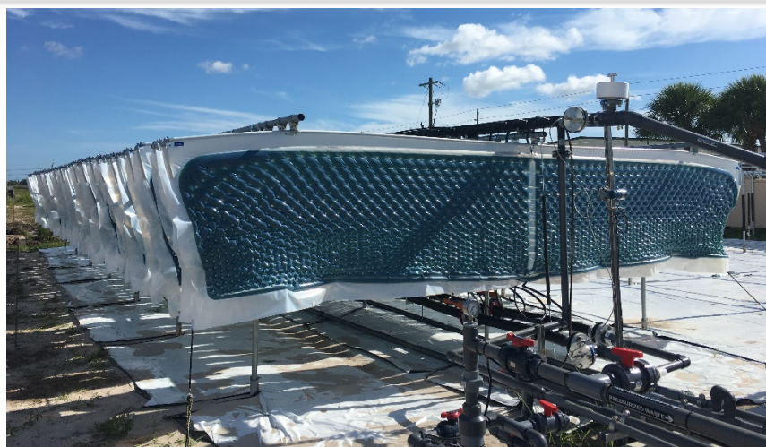
Figure 8-1: 6,000-L PBR Array fully inoculated with AB1166 culture. PBR faces are in a north-south orientation.
