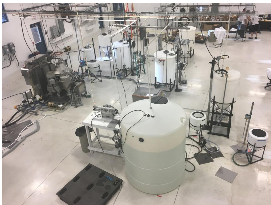
Figure 7-6. DEMO PC extraction and purification line in Algenol Engineering High Bay.
