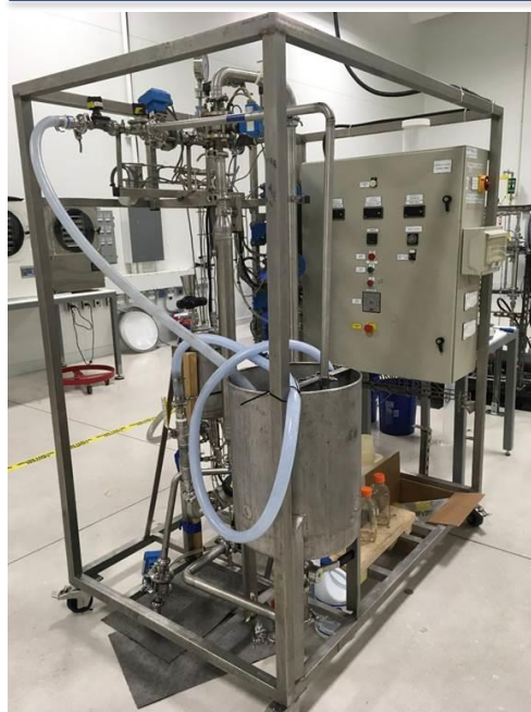
Figure 7-12. Ceramic cross-flow microfiltration (MF) unit leased from Novasep that is analogous to the commercial design.
