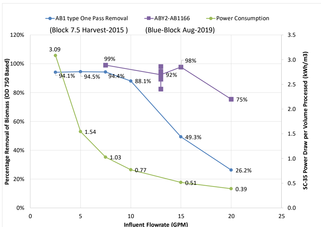
Figure 8-13: Power consumption from Algenol dewatering tests using a GEA SC-35 continuous centrifuge. Tested strains were Cyanobacterium sp. AB1 and AB1166.
