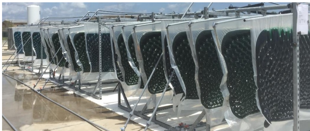
Figure 4-1. Automated airlift system showing the six 3-PBR units. Each set of airlifts is flanked by a dye bag at the east and west end, with one dye bag separating the duplicate airlifts.
