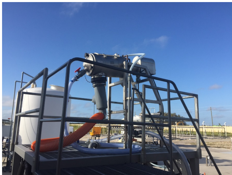
Figure 6-4. Russel Finex Liquid Solid Separator Installed on Platform at DEMO
