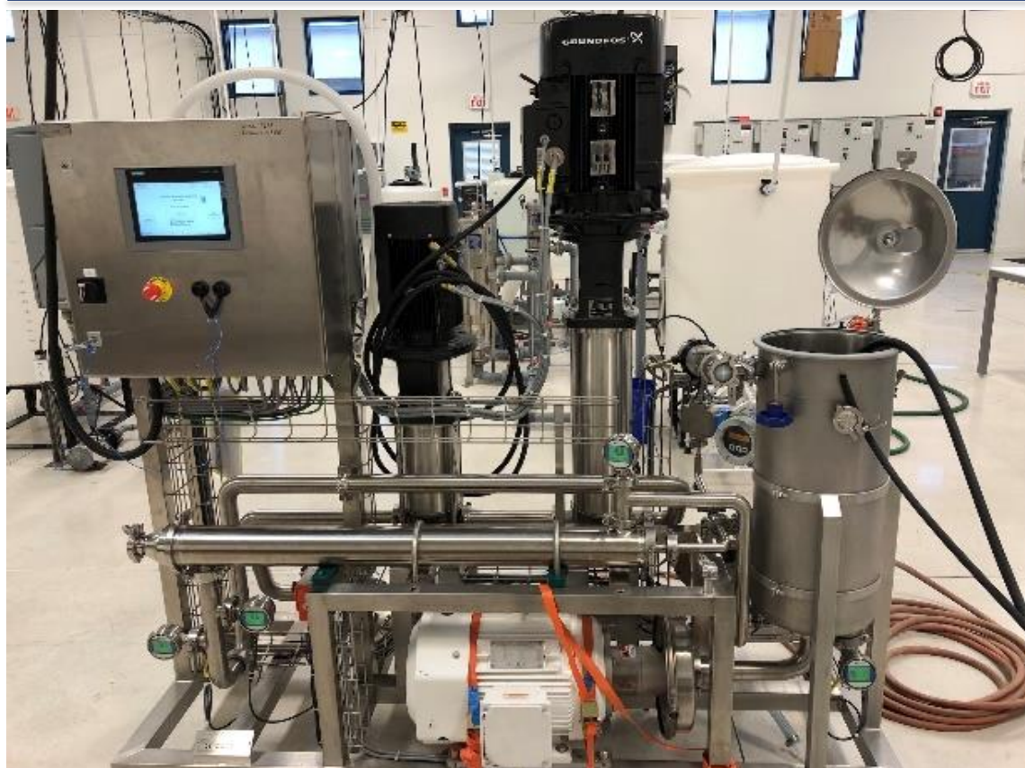
Figure 7-13. Alfa Laval ultrafiltration (UF) pilot system used at DEMO.
