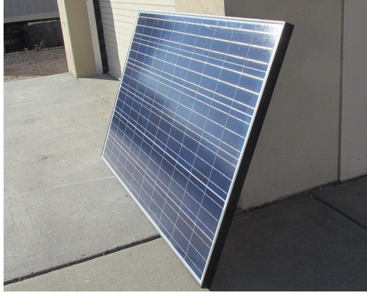
Figure 2-9. Module setup on exterior wall for I-V curve trace measurements.
