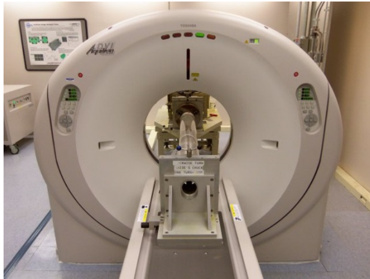
Figure 23: A 16 slice Aquillion CT scanner.
