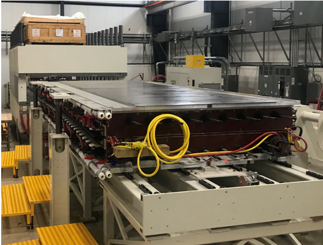
Figure 77. Picture of tooling stack-up and simulated part ready for loading into the restraint for processing
