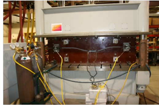
Figure 20. Tooling and resistance welded aluminum bladders are ready to begin the forming of the bladder and subsequent stiffener to panel co-consolidation
