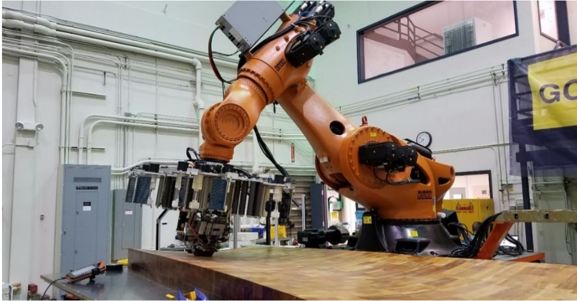
Figure 53. Picture of 1/2" wide tape head installed onto the robot performing a mechanical test showing tape laying course travel over the demo skin lay-up tool
