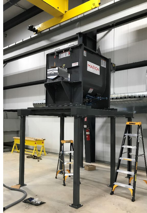
Figure 64. Depiction and picture of the ceramic mixer and tool casting system
