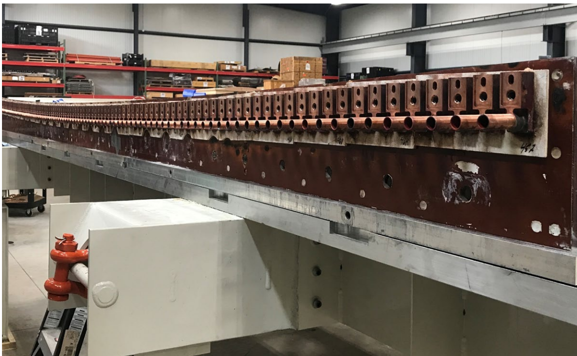
Figure 69. Picture of copper coil connectors after brazing
