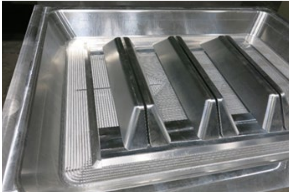
Figure 9. Machined aluminum co-consolidation tooling
