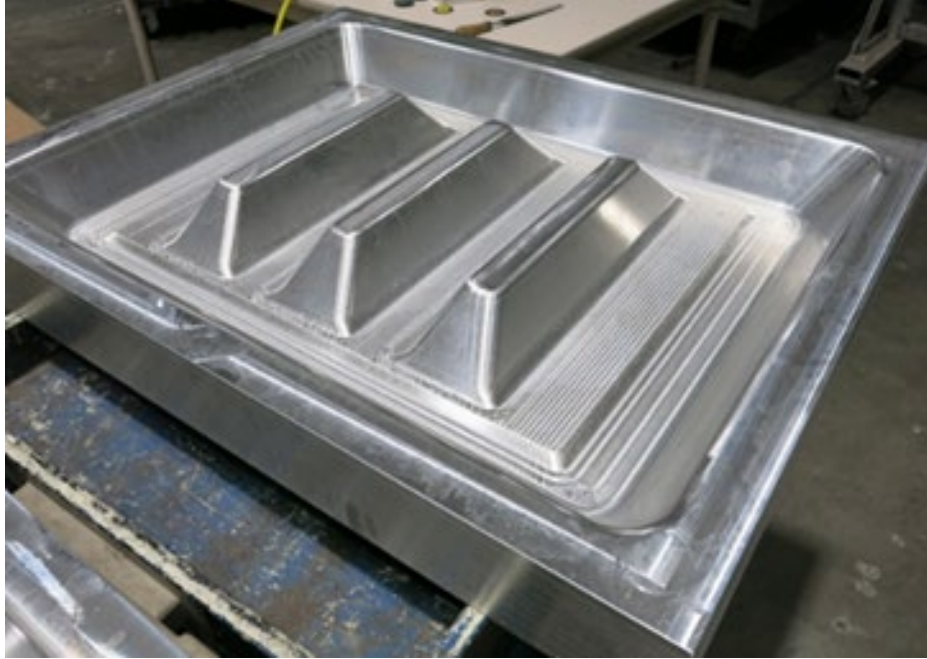
Figure 7. Forming tool for the flat blade stiffened panel aluminum consolidation bladder
