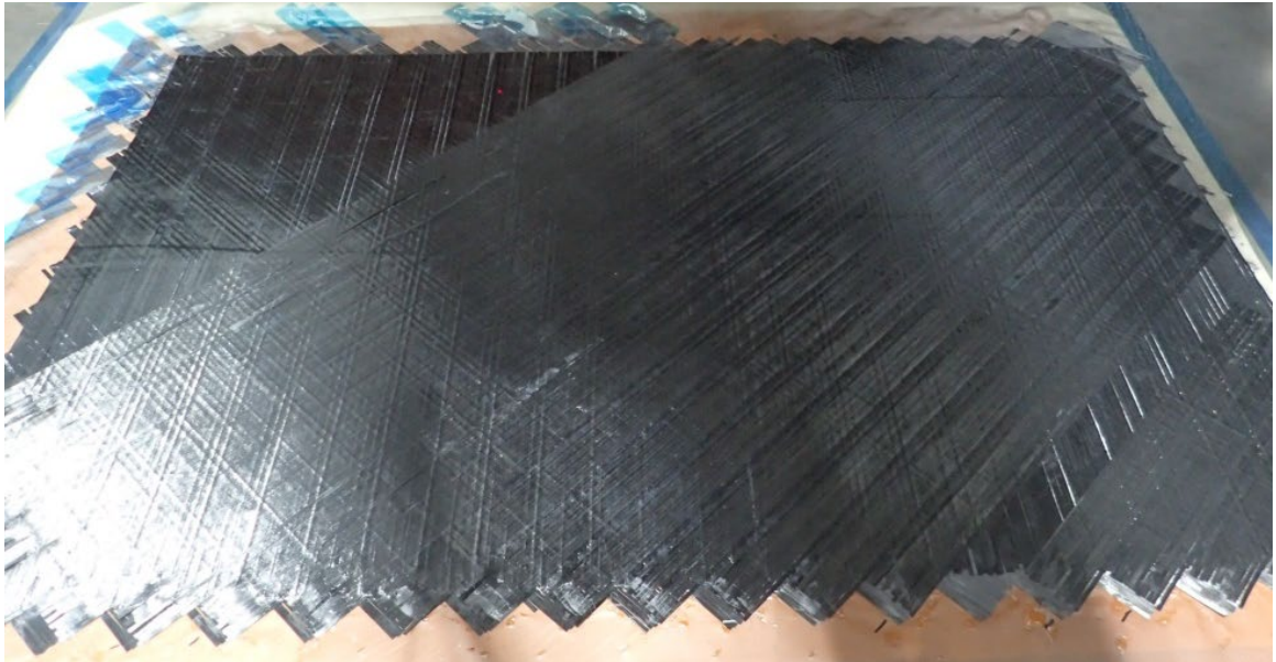
Figure 29. Picture of the flat panel skin lay-up depicting a 45 degree ply
