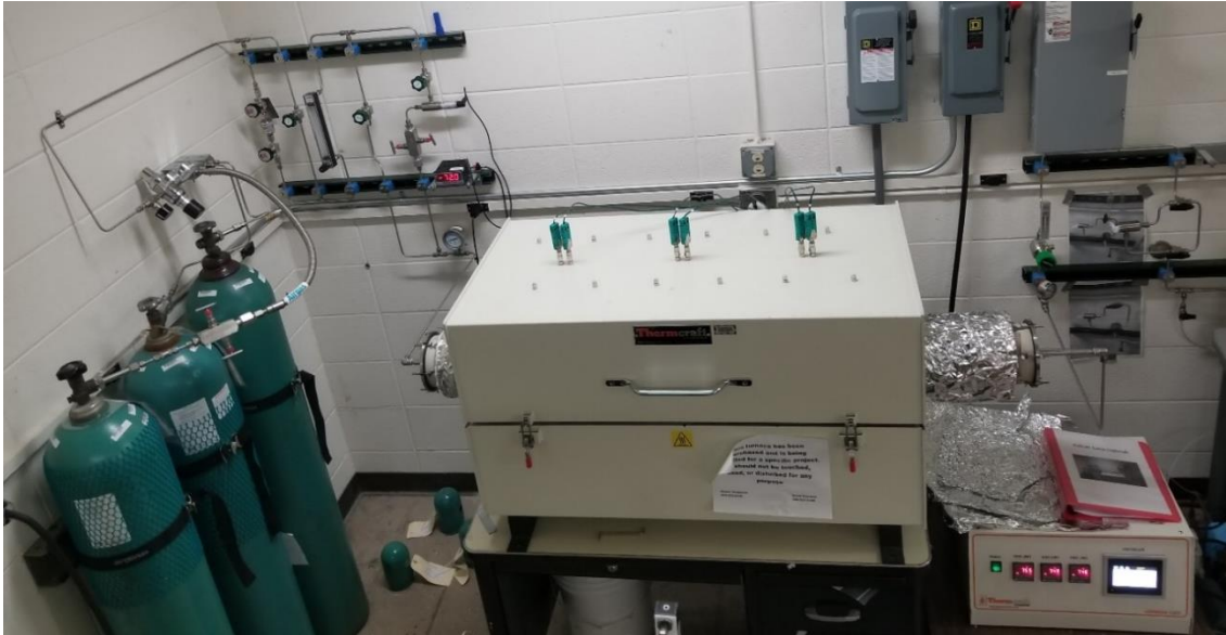
Figure 9: Photograph of the once-through helium loop used in this research.
