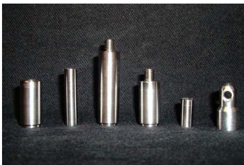
Figure 9: Neutron Isotopic Sources are Typically Encapsulated in Stainless Steel or Similar Materials.
