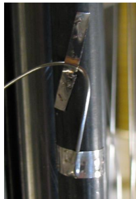
Figure 2.8 Typical TC attachment to heater rod.
