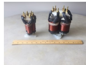
Fig. 8. Line side (right) and inverter side (left) inductors.
