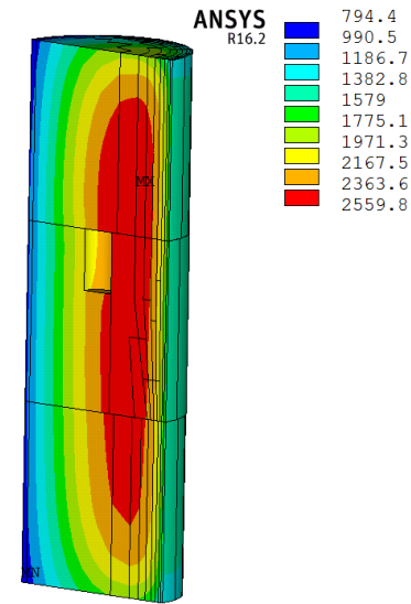
Fig. 7. Pellet temperature profile ( ^{\circ}\text{C} ) at EOC 3
