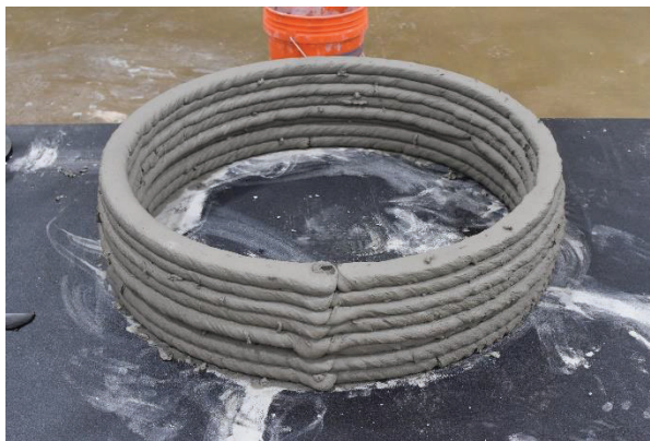
Figure 12. The first test print of the SkyBAAM system: an eight-layer circle
