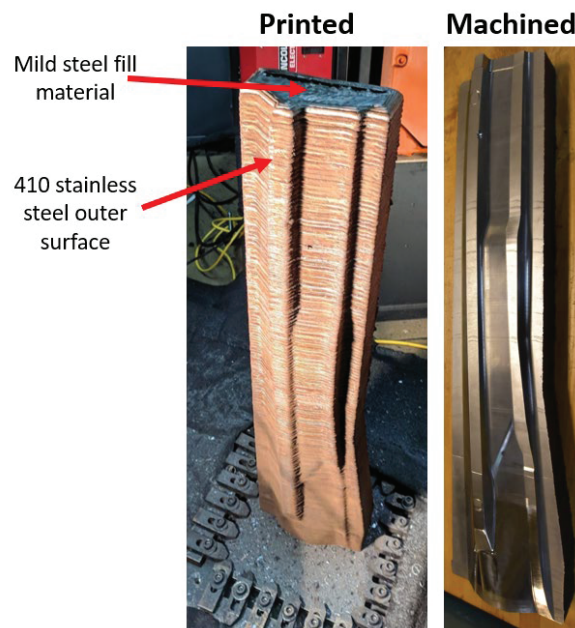
Figure 11. Multi-material stamping tool with an outer surface of stainless steel and an inner core of mild steel
