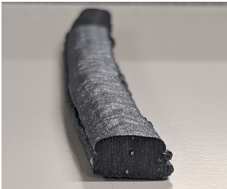
Figure 5: Cross Section of beads with wire
