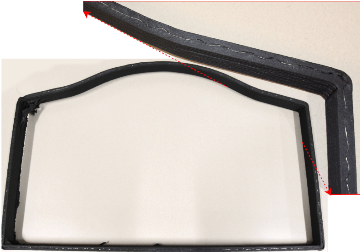
Figure 6: Single Bead Part Printed with Tamper
