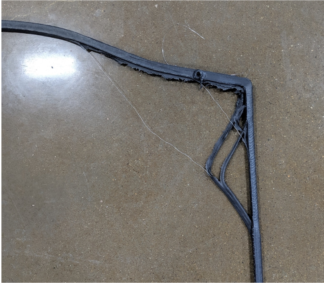
Figure 3: Failed part from motor running too slowly
